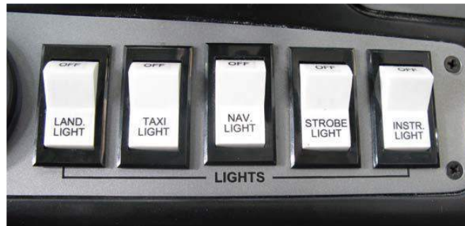
Figure 11. – Lights switches panel
